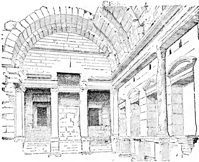
STONE CUTTING, FIG. 6: BARREL VAULT OF PECULIAR CONSTRUCTION; NYMPHÆUM AT NIMES, SOUTH OF FRANCE; ROMAN IMPERIAL WORK.
